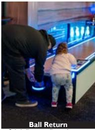
Side ball return allows players to watch the ball being returned and allows operators ease of access to ball return. Safety is key so there is no pinch point at pickup.
